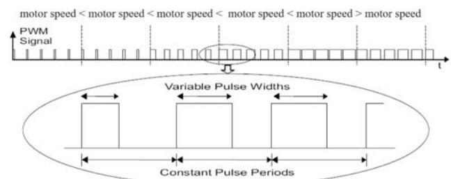
Fig.1. Pulse width modulation waveforms
