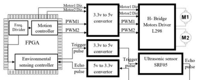
Fig. 5 Mobile robot controller main architecture
