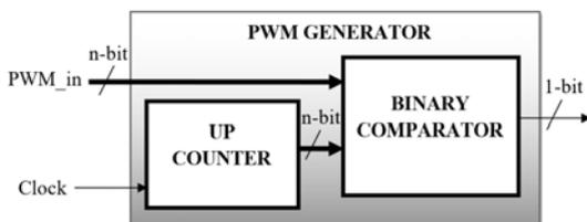
Fig. 7 PWM generator architecture
