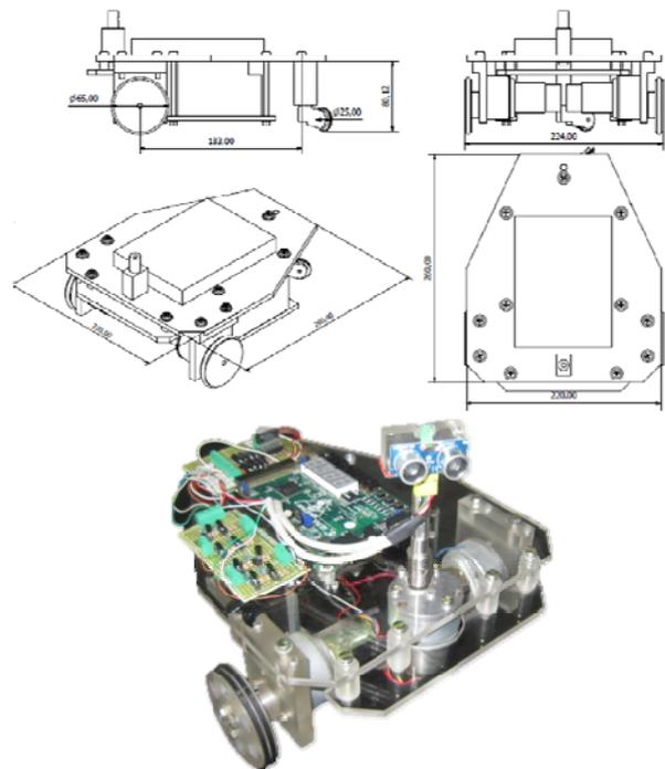
Fig.4. Mechanical design of the mobile robot
