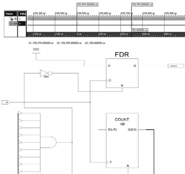
Fig. 6 Frequency divider test and RTL schematic
