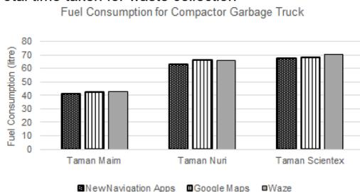
Fig.7. Fuel consumption for the compactor garbage truck
