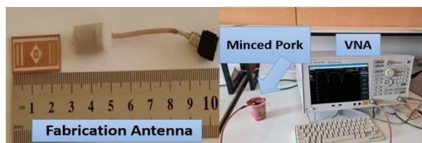
Fig 11. Photographs of the Fabrication proposed fractal capsule Antenna.
