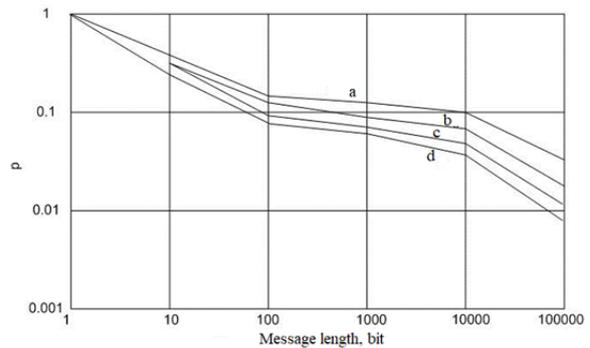
Fig. 8. Probability of error-free transfer of information depending on the mode and amplitude of transfer: a – bipolar mode, 12 V; b – bipolar mode, 5 V; c – unipolar mode, 12 V; d – unipolar mode, 5 V.
