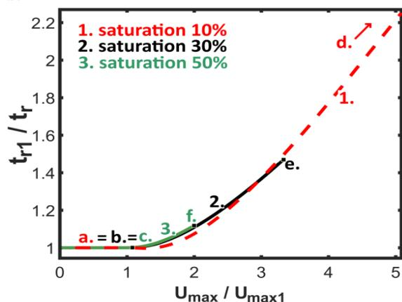
Fig.6. Relative control quality indicator for  $t_r$  for saturation  $U_{max1}=10\%U_{max}, U_{max1}=30\%U_{max}$  and  $U_{max1}=50\%U_{max}$
