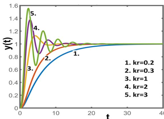
Fig.8. Output signal  $y(t)$  for various values of  $k_r$  for example 2
