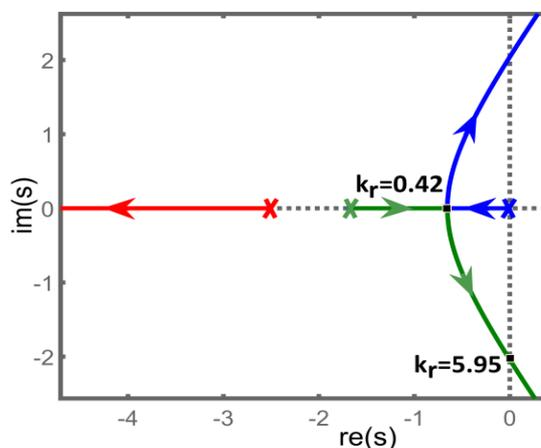
Fig.7. Root locus plot for the example 2
