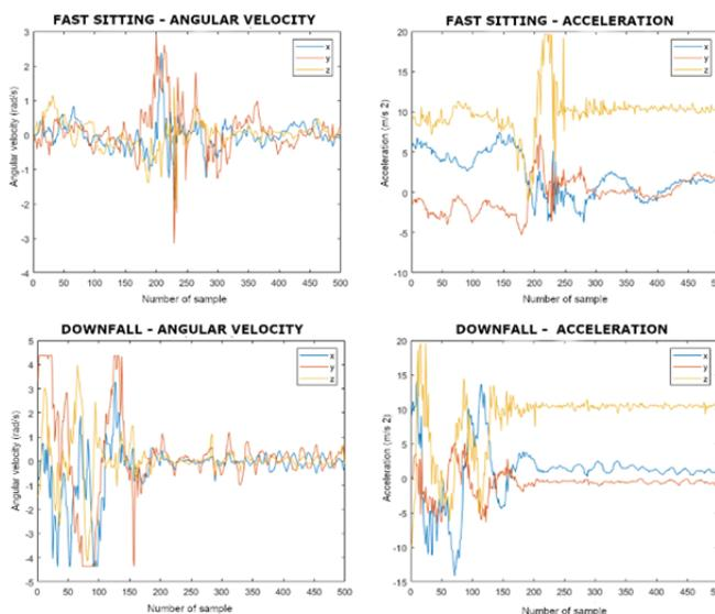
Fig. 6. MPU6050 sensor indications while fast sitting and downfall
