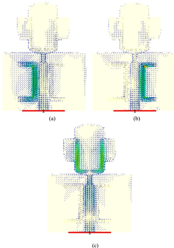
Fig. 9. Simulated surface current distribution of proposed UWB antenna of Antenna C1 at (a) 5.2 GHz, (b) 5.8 GHz and (c) 8.0 GHz
