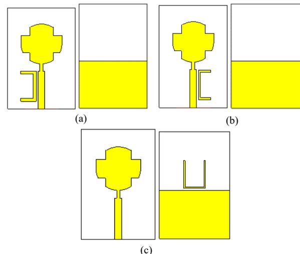
Fig. 2. Schematic diagram of the development for proposed monopole antenna with U-shaped element (a) Antenna B1 (b) Antenna B2, (c), Antenna B3
