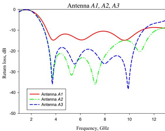
Fig. 4. Return loss of the for the proposed monopole antenna of Antenna A1, Antenna A2 and Antenna A3
