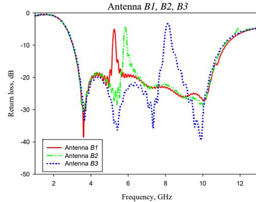
Fig. 5. Return loss of the for the proposed monopole antenna of Antenna B1, Antenna B2 and Antenna B3
