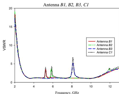
Fig. 8. VSWR of the for the proposed monopole antenna of Antenna B1, Antenna B2, Antenna B3 and Antenna C1
