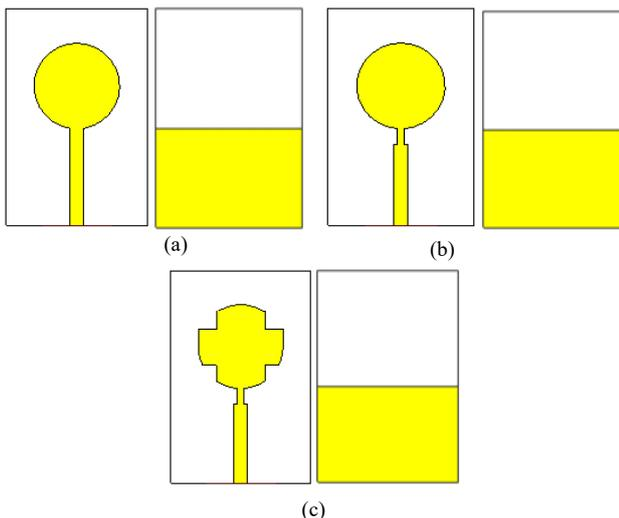
Fig. 1. Schematic diagram of the development for proposed monopole antenna (a) Antenna A1 (b) Antenna A2, (c), Antenna A3
