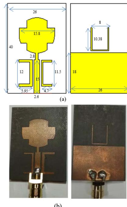
Fig. 3. Schematic diagram of the development for proposed monopole antenna of Antenna C1 with combined three U-shaped elements, (a) simulation, (b) fabricated
