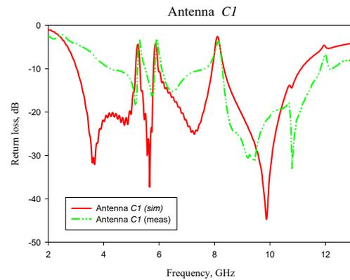
Fig. 6. Return loss of the for the proposed monopole antenna of Antenna C1 (simulation vs measurement)
