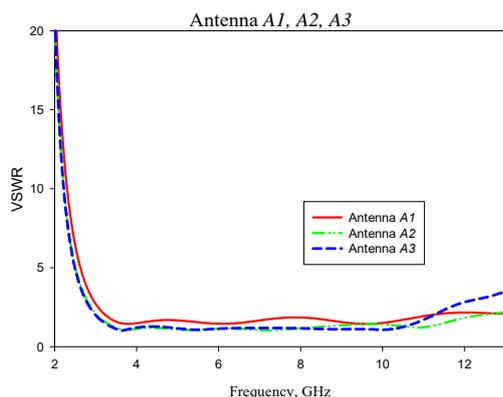
Fig. 7. VSWR of the for the proposed monopole antenna of Antenna A1, Antenna A2 and Antenna A3
