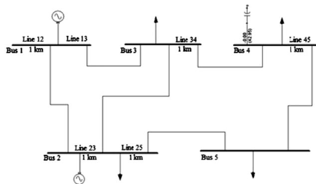
Fig. 6. 5-bus system layout under line 2-4 outage with shunt capacitor at bus number 4
