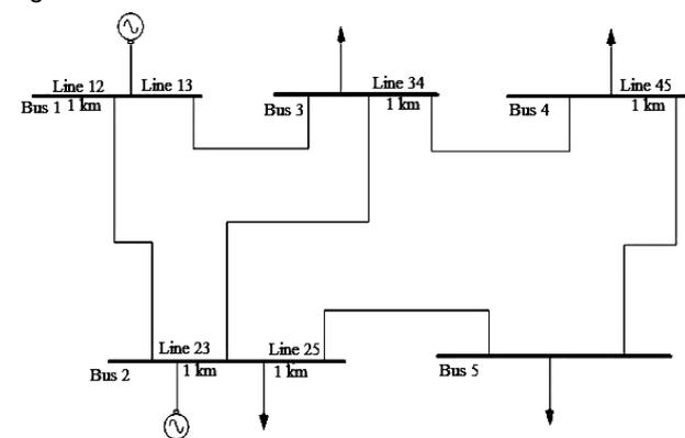
Fig. 5. The 5-Bus system layout under line 2-4 outage
