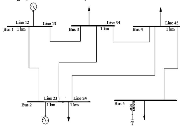
Fig. 8. The 5-bus system layout under line 2-5 outage with shunt capacitor at bus number 5
