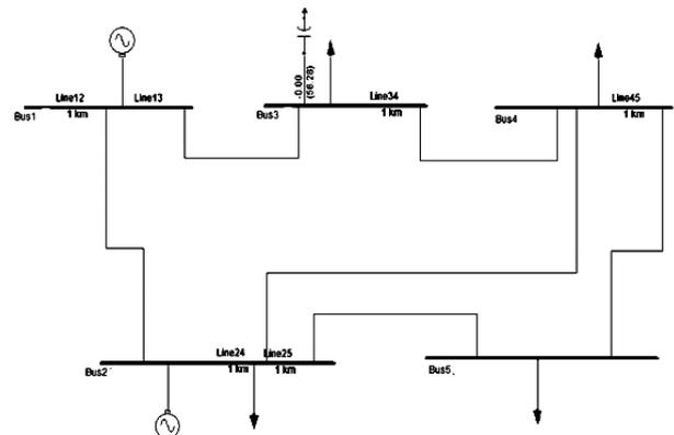
Fig. 4. The 5-bus system layout under line 2-3 outage with shunt capacitor at bus number 3
