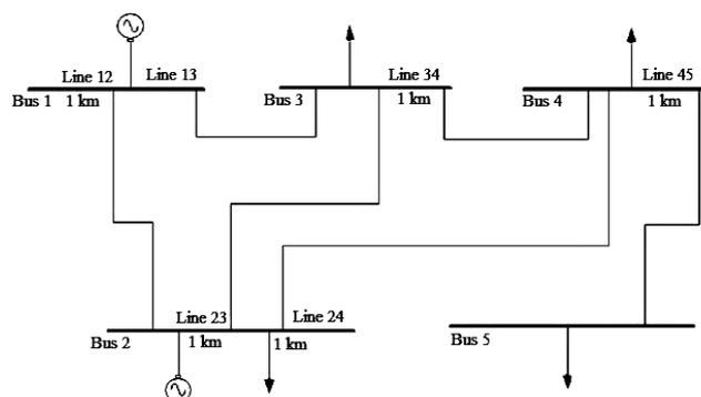
Fig. 7. 5-bus system layout under line 2-5 outage
