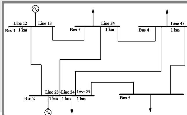
Fig. 1. The 5-bus system base case layout
