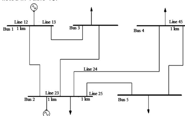
Fig. 9. The 5-bus system layout under line 2-5 outage with shunt capacitor at bus number 5
