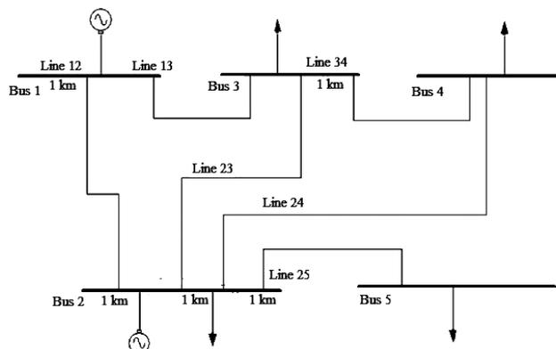
Fig. 10. The 5-bus system layout under line 4-5 outage
