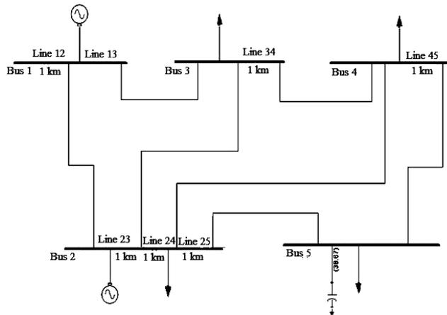
Fig. 2. The 5-bus system with shunt capacitor at bus number 5
