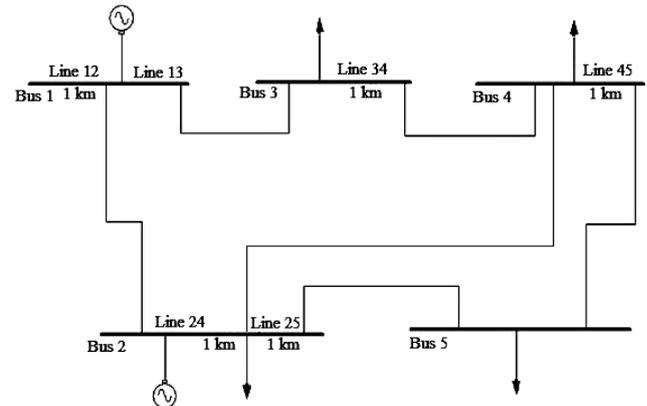
Fig. 3. The 5-bus system layout under line 2-3 outage
