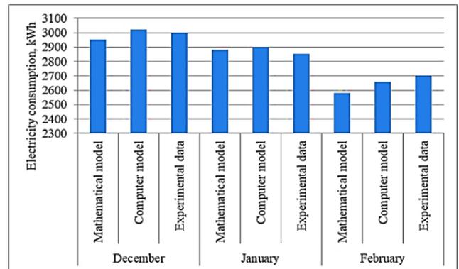
Fig. 9. Results of comparing simulation of power consumption with experimental data
