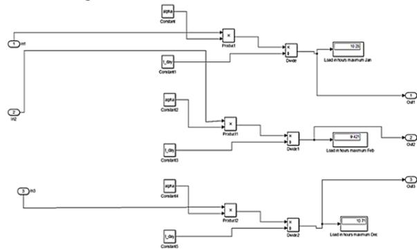
Fig. 8. Block for simulating load during peak hours
