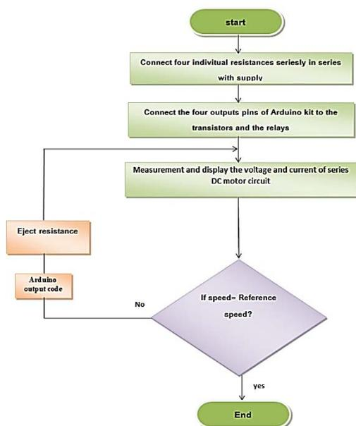
Fig.3. Flowchart of series DC motor based Arduino.
