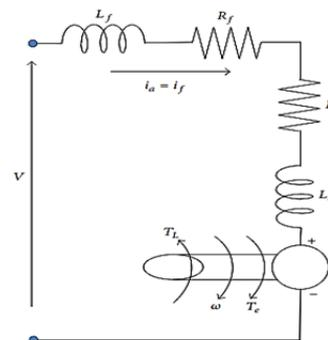
Fig.2. A DC motor in series electrical diagram.
