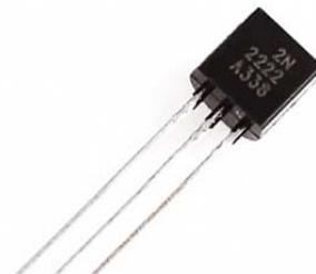
Fig.5. NPN bipolar transistor.
