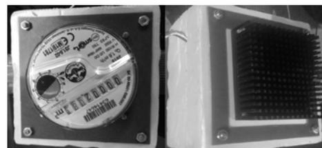
Fig. 2. Laboratory set-up for testing heat energy harvester based on cold tap water meter
