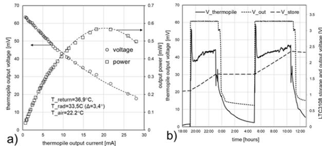
Figs. 7. Performance of the thermoelectric energy harvester operated on the return path of the domestic heating system: a) current-voltage and current-power characteristic at the mid-temperature difference (3.4°C), b) daily record of system voltages.
