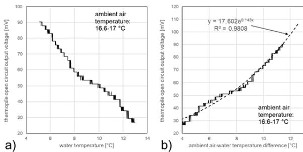
Fig. 3. Experimental record of the thermopile open circuit output voltage as a function of: a) supply water temperature, b) ambient air and supply water temperature difference.
