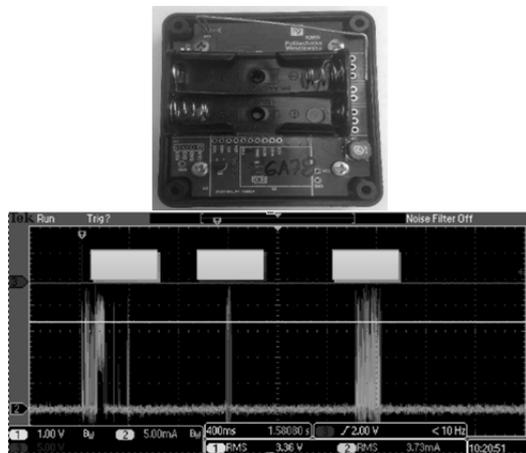
Fig. 1. Battery-powered autonomous sensor platform with environmental multiparametric sensor and LoRaWAN communication: a) prototype interior view, b) changes in battery voltage (purple curve), supply voltage (yellow curve) and supply current (green curve) during one measurement and data transmission cycle (7.2 V battery voltage).
