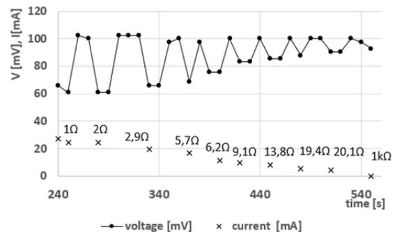
Fig. 4. a) Experimental record of the measured voltage and current values for a cell loaded with a resistance of 1 ohm up to the stabilized temperature conditions of the water meter housing (heat sink),
