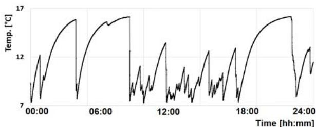
Fig 5. Exemplary daily record of water temperature in the building supply pipe
