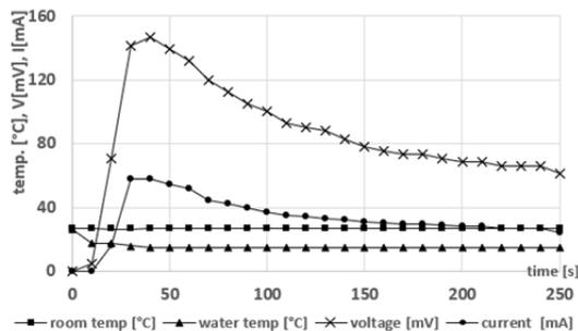
Fig. 4. b) The value of the measured voltage and current for a cell loaded with a resistance in the range 1  $\Omega$ - 1 k $\Omega$ .
