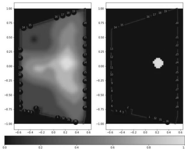
Fig.5. Resulting image reconstruction performed by 32-element RTI system for unfiltered (left) and filtered (right) matrix
