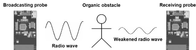
Fig.2. The principle of RTI technology in the context of in-building navigation
