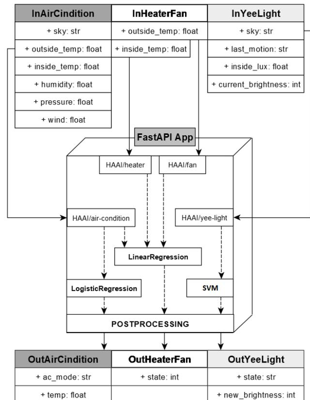
Fig.9. Scheme/algorithm of ML activities applied to the building under test
