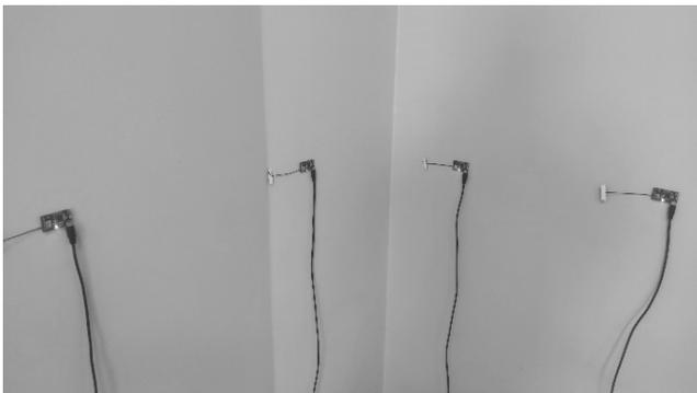
Fig.7. Fragment of a loop of hybrid 2.4 GHz radio probes girdling the test room
