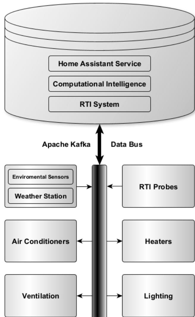
Fig.1. Graphical representation of the management system structure using computational intelligence and RTI algorithms
