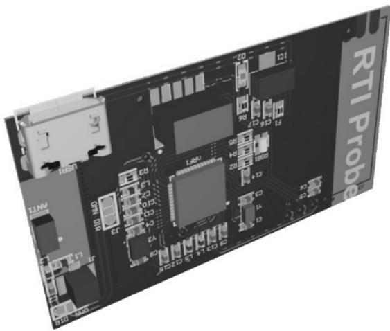
Fig.6. 3D visualization of the PCB of the 2.4 GHz radio probe
