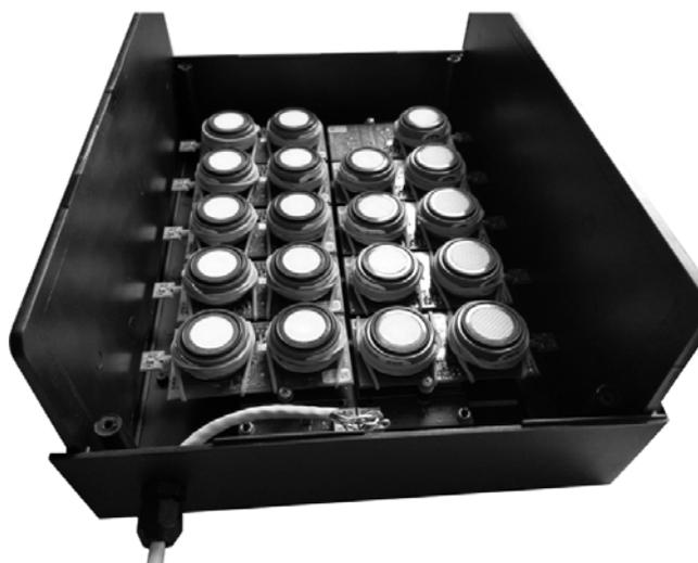
Fig. 7. The measurement set containing 10 modules with sensors NO2- B43F and SO2-B4
