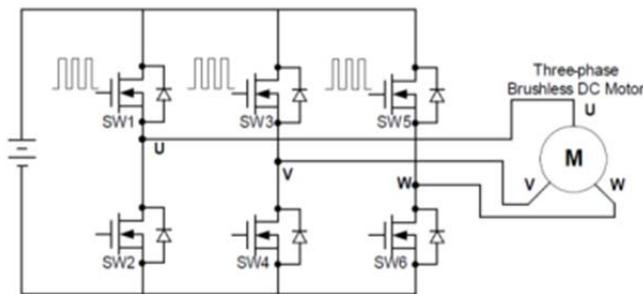
Fig 3. 3 Phase Inverter Circuit
