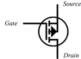
Fig 2. MOSFET Circuit
