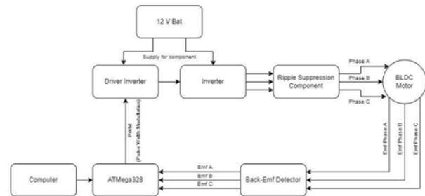
Fig 7. Control Circuit System Schematic
