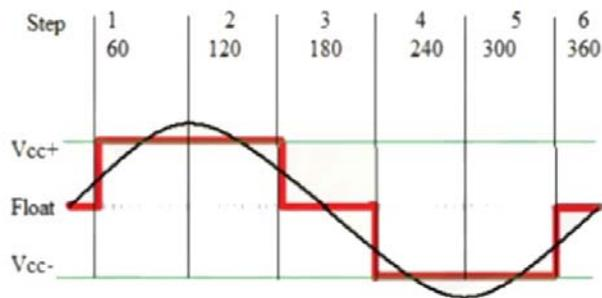
Fig 5. Determination of the Six-Step Method
