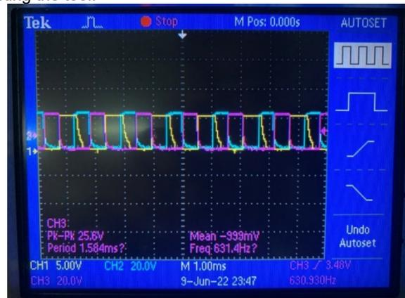
Fig 18. 3-Phase Wave Without Ripple Suppression
