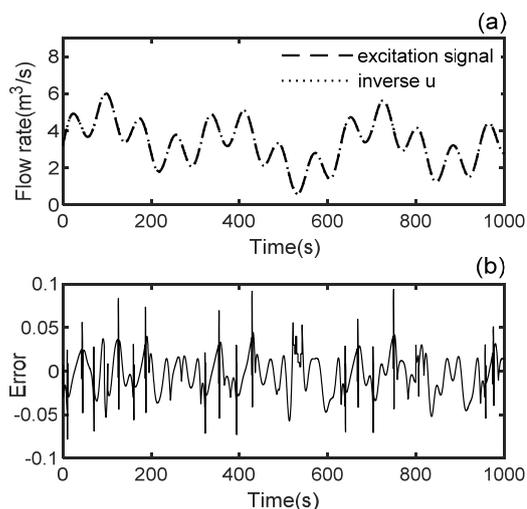
Fig.8. (a) Comparison of the system input and the inverse controller output (b) error of the constructed inverse controller
