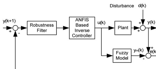
Fig.9. Proposed internal model control structure
