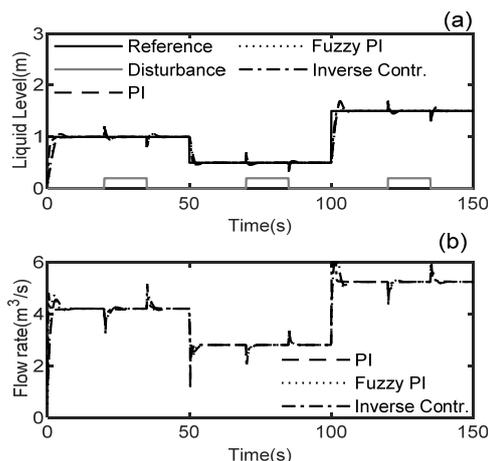
Fig. 14. a) Comparison of the system responses under the output disturbance condition b) control signals
