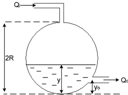
Fig.1. Spherical tank system
