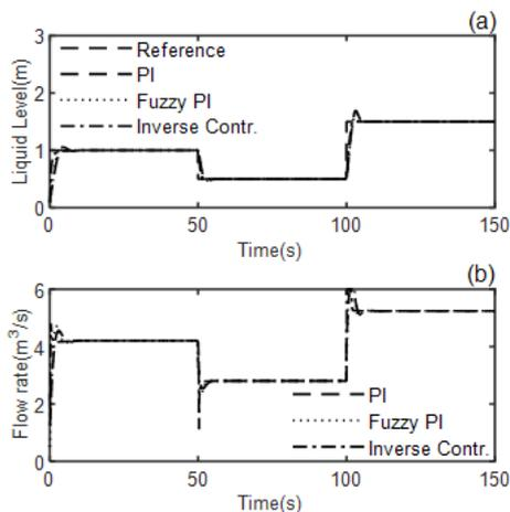
Fig. 13. a) Comparison of the system responses under the set point variation condition b) control signals
