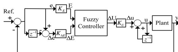
Fig.10. Structure of the fuzzy PI controller
