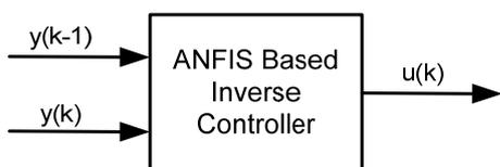
Fig.6. Input-output configuration of the ANFIS based inverse controller
