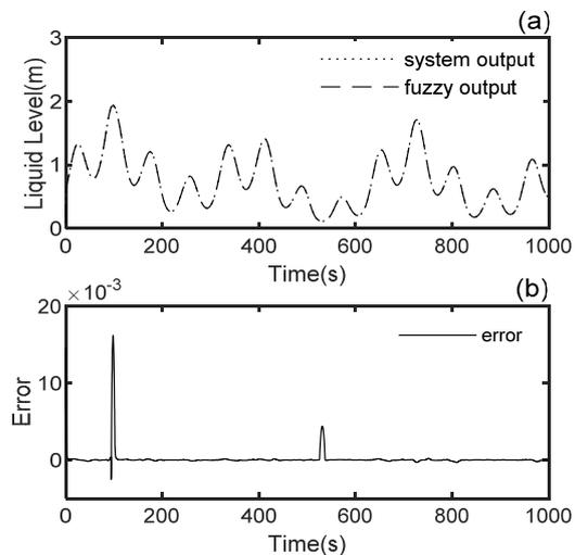
Fig.5. (a) Comparison of the system output and the fuzzy model output (b) modeling error of the constructed fuzzy model
