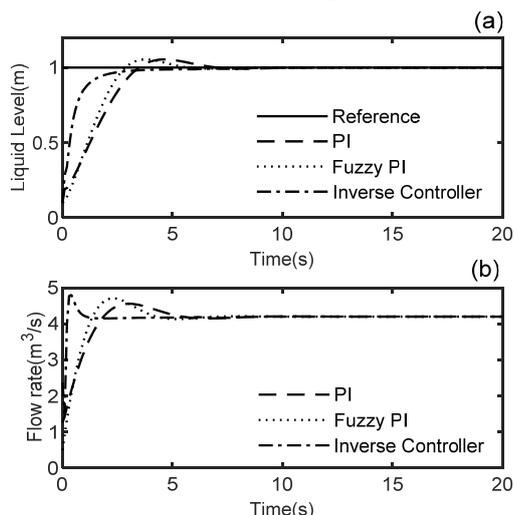
Fig. 12. a) Comparison of the system responses for unit reference signal b) control signals
