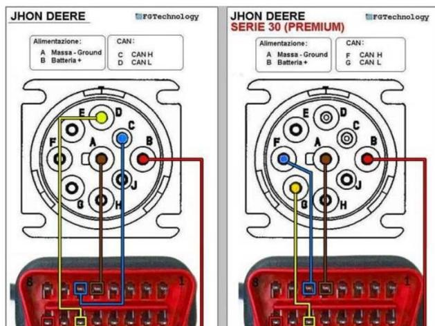
Fig. 6. Connection diagram of EDL and OBDII socket [11].
