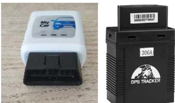
Fig. 4 Signal transmission devices from the tractor information system
