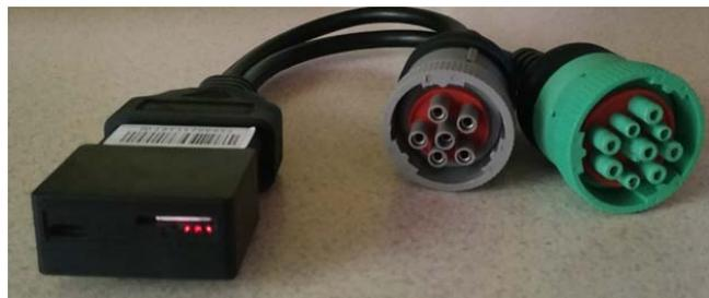
Fig. 7. Locator with adapter for John Deere tractor communication socket
