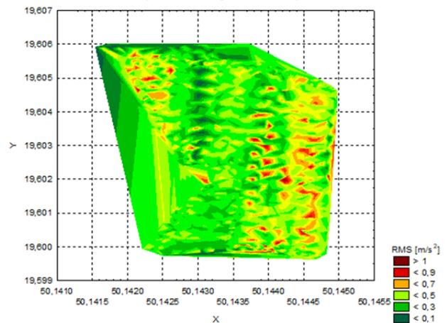
Fig. 9. Variation of the rms value of vibration accelerations (RMS) measured on the seat of a farm tractor for the vertical direction of interaction within the experimental field.
