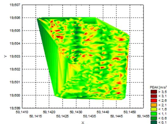
Fig. 3. Variation of the peak value of vibration acceleration (PEAK) measured on the seat of an agricultural tractor for the vertical direction of interaction within the experimental field.
