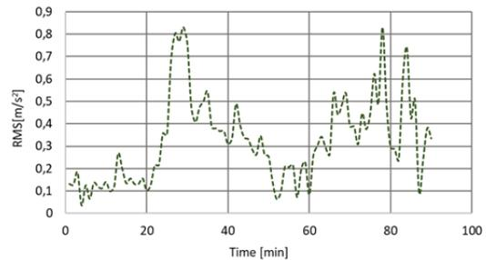
Fig. 8. The rms value of vibration acceleration ( $\text{RMS}_{\text{MAX}}$ ) measured on the seat of an agricultural tractor for the vertical direction of interaction
