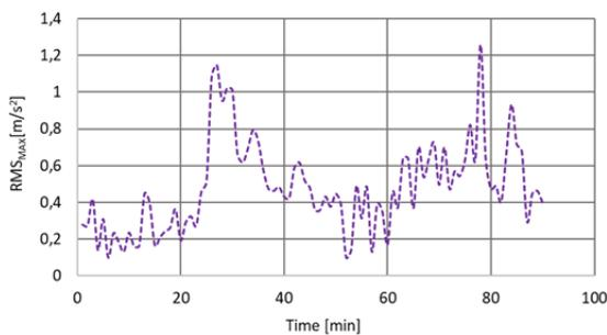
Fig. 6. The maximum rms value of vibration acceleration ( $\text{RMS}_{\text{MAX}}$ ) measured on the seat of an agricultural tractor for the vertical direction of interaction
