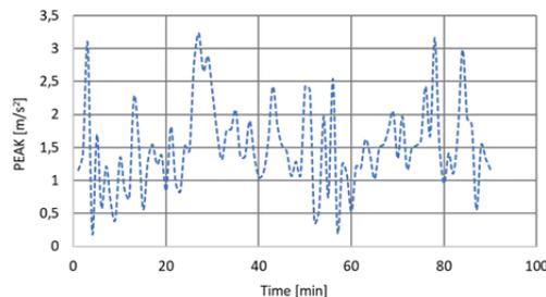
Fig. 2. Peak value of vibration acceleration (PEAK) measured at the seat of the agricultural tractor for the vertical direction of impact
