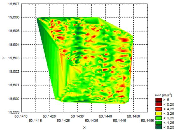
Fig. 5. Variation of the inter-peak value of vibration acceleration (P-P) measured on the seat of an agricultural tractor for the vertical direction of interaction within the experimental field.
