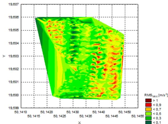
Fig. 7. Variation of the maximum rms value of vibration acceleration ( $\text{RMS}_{\text{MAX}}$ ) measured on the seat of an agricultural tractor for the vertical direction of impact within the experimental field
