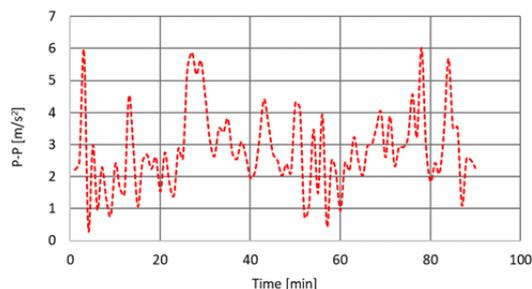
Fig. 4. The inter-peak value of vibration acceleration (P-P) measured on the seat of an agricultural tractor for the vertical direction of interaction
