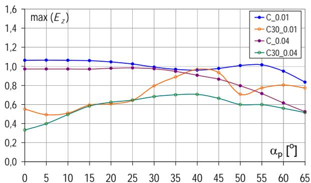
Fig.5. Characteristics of changes in the maximum value of the field intensity  $\max(E_z)$  as a function of the angle of incidence of the electromagnetic wave
