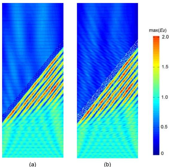
Fig.6. Envelopes of the maximum value of the  $E_z$  component in the area under consideration, at  $\alpha_p = 60^\circ$  for models: (a) C\_01, (b) C30\_01
