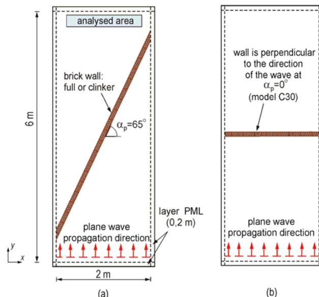
Fig. 3. Model geometry for the angle of incidence of an electromagnetic wave: (a) maximum angle, i.e. 65°, (b) minimum angle, i.e. 0°
