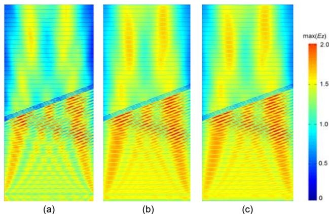
Fig.4. Modelled PML layer tests: a) PML=0.1 m, b) PML=0.2 m, c) PML=0.3 m
