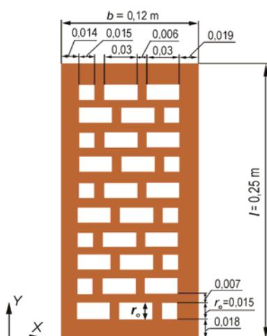
Fig. 2. Geometrical sizes of brick with hollows (B30)
