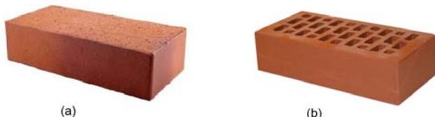
Fig. 1. Two models of analysed bricks: a) solid brick; b) brick with 30 holes
