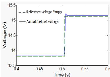
Fig. 9 Fuel cell voltage under varying operating conditions
