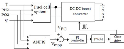
Fig. 8 Overall proposed MPPT system
