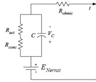
Fig.2. PEMFC Equivalent dynamic electrical circuit
