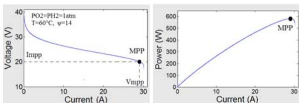
Fig. 5 500-W BCS stack electrical output characteristics
