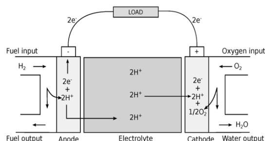
Fig.1. Fuel cell principle [4]
