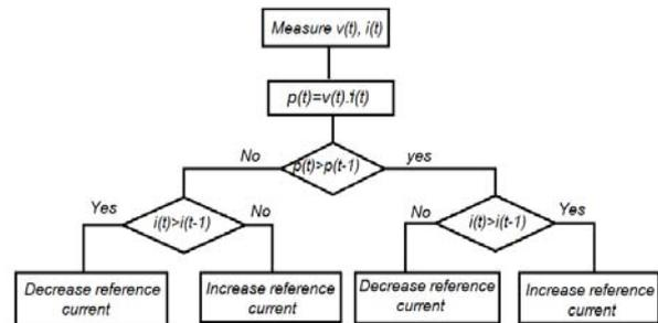
Fig. 10 Perturb and observe (P&O) MPPT algorithm
