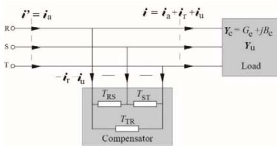
Fig. 7. A load with a reactance balancing compensator.
