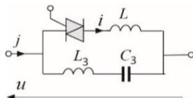
Fig. 8. A TSI with a filter of the 3<sup>rd</sup> order harmonic.
