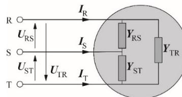
Fig. 5. An equivalent circuit of a three-phase load.
