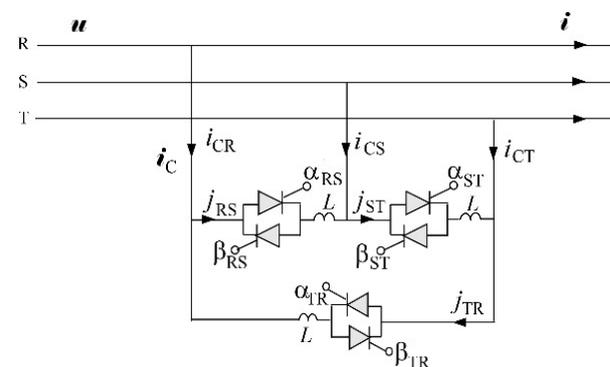
Fig. 10. A balancing compensator with asymmetrically switched thyristors.
