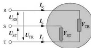
Fig. 6. An equivalent circuit of a three-phase load.
