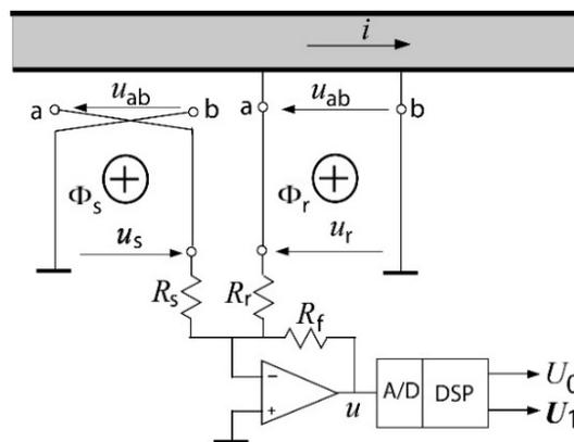
Fig. 2. A DC current sensor.
