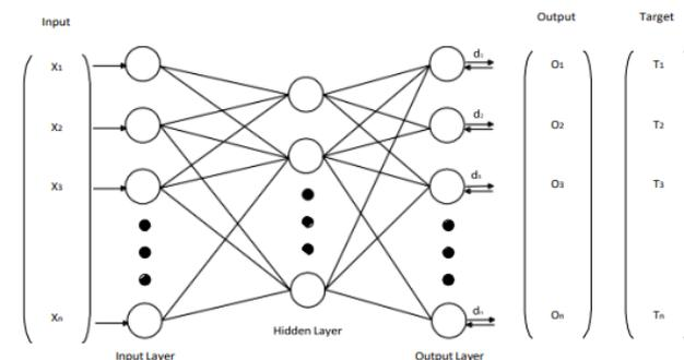
Fig. 2. Backpropagation network architecture[12]
