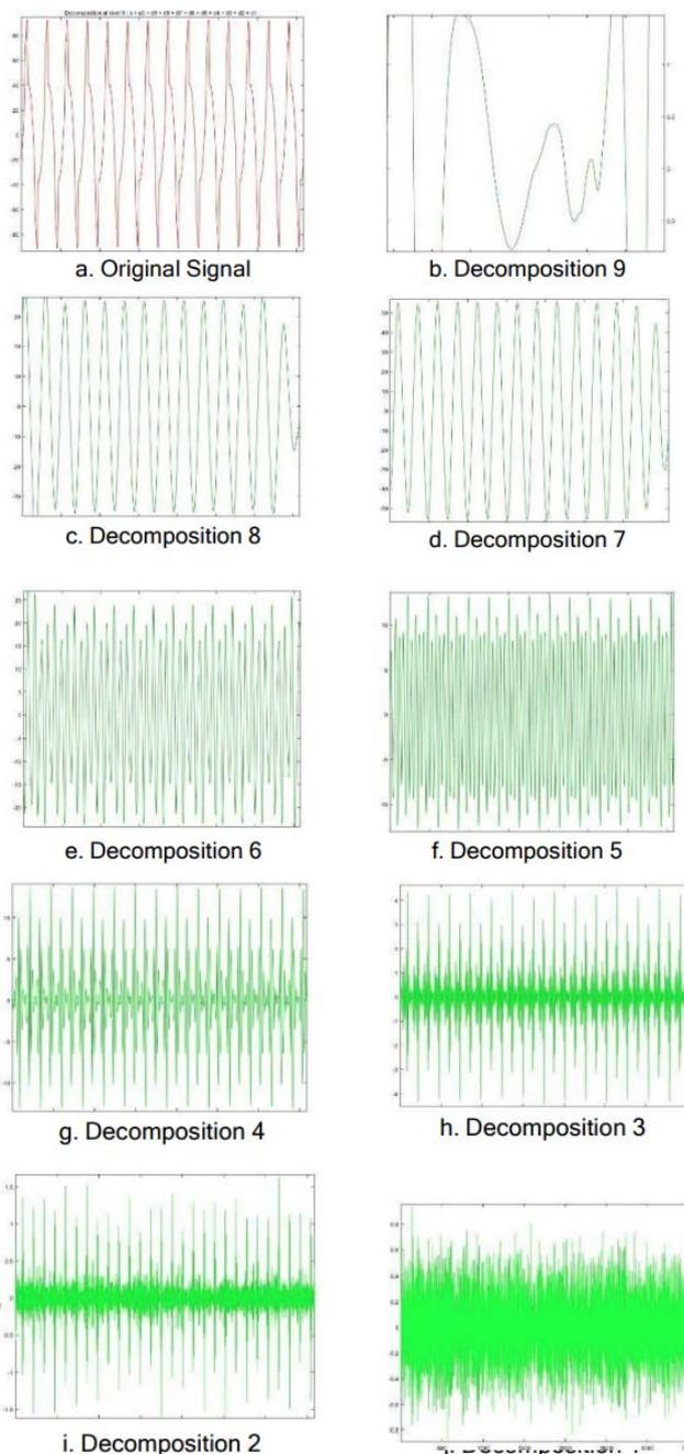
Fig. 6. The result of wavelet decomposition on transformer TR-1
