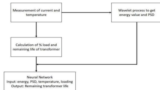
Fig. 3. Block diagram of research stages
