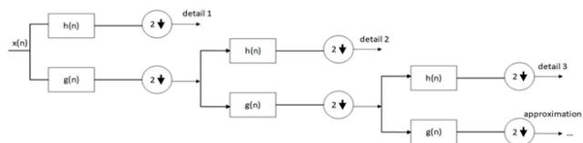
Fig. 1. Wavelet decomposition tree
