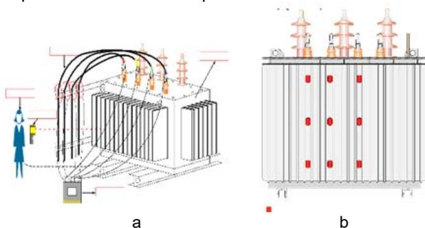
Fig. 4. (a) Sketch of transformer current measurement (b) Sketch of transformer temperature measurement
