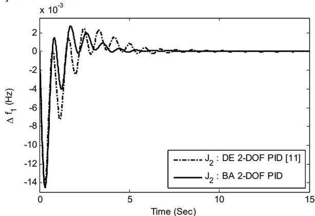
Fig.6. Frequency deviation of area-1 for 1% change in area-1 with ITSE objective function.
