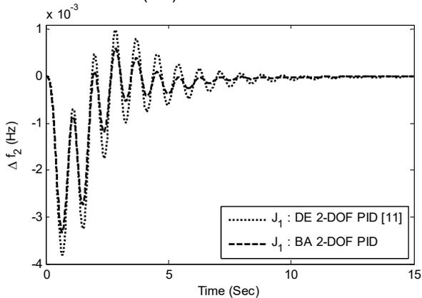
Fig.4. Frequency deviation of area-2 for 1% change in area-1 with ISE objective function.
