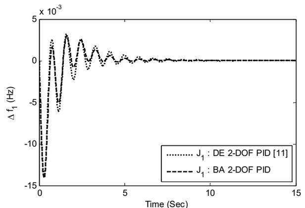
Fig.3. Frequency deviation of area-1 for 1% change in area-1 with ISE objective function.
