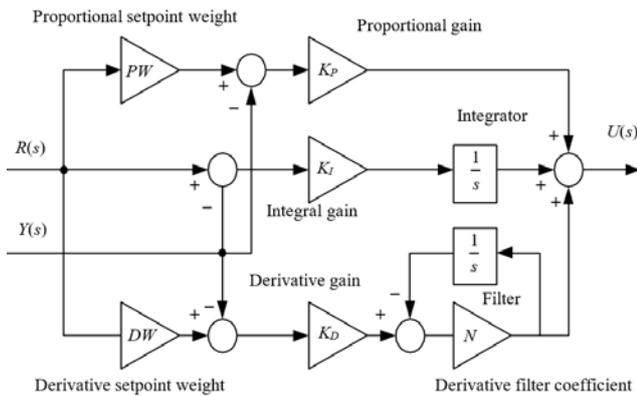
Fig.2. Two degrees of freedom (2-DOF) PIDcontroller
