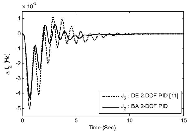
Fig.7. Frequency deviation of area-2 for 1% change in area-1 with ITSE objective function.
