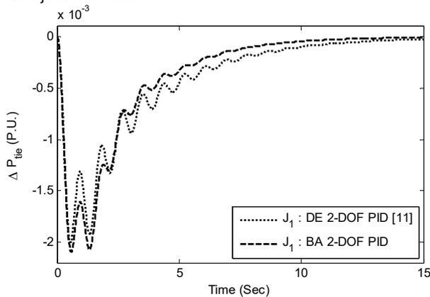
Fig.5. Tie line power deviation for 1% change in area-1 with ISE objective function
