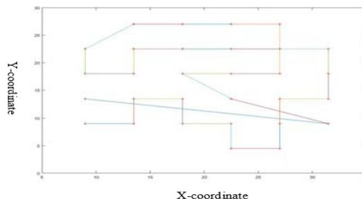
Fig 3. Distribution of node sensors as a PEGASIS network
