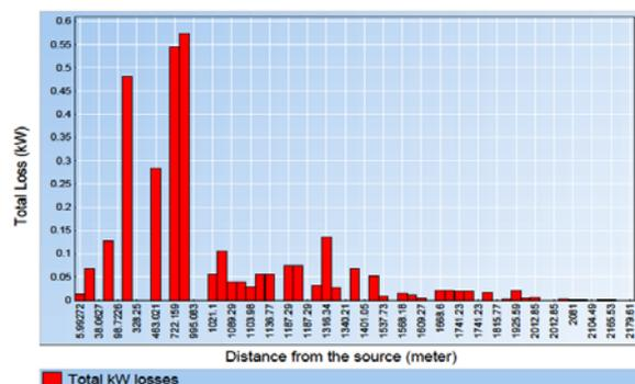
Fig.7. Total losses of Al-qethara 33 kV feeder
