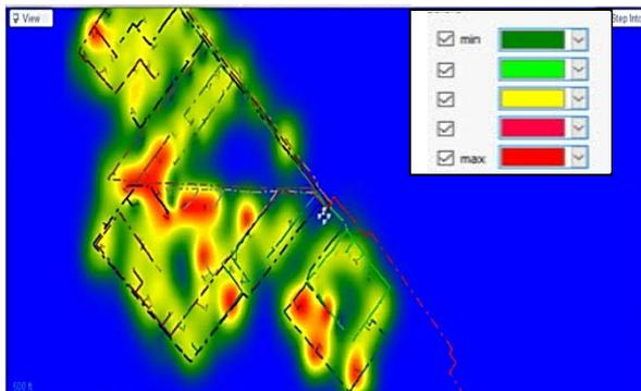
Fig.3.b. Load density of 5-mail proposed 33/0.416 kV network after re-location of 33/0.416 kV distribution transformers using CYME
