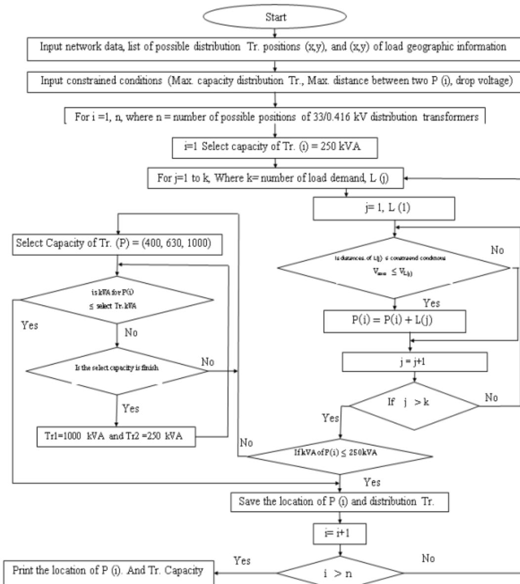
Fig.1. Flow chart representing the methodology of optimal location and capacity of distribution transformers
