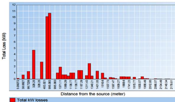
Fig.6. Total losses of Al-qethara 11 kV feeder
