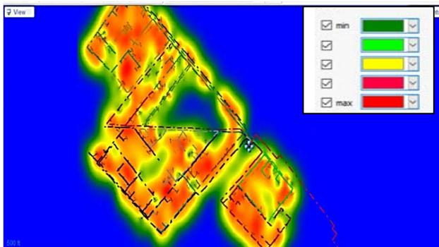
Fig.3.a. Load density of 5-mail proposed 33/0.416 kV network before re-location of 33/0.416 kV distribution transformer using CYME
