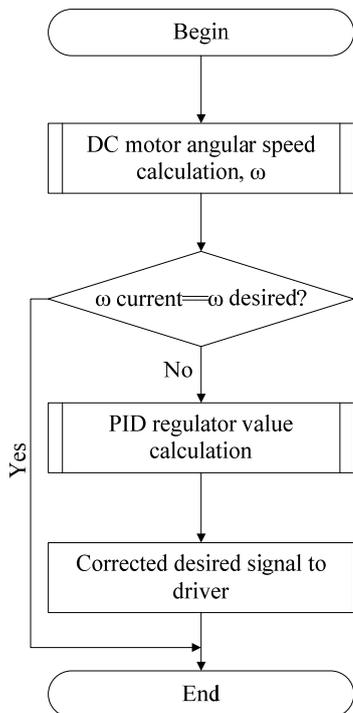
Fig. 5. Algorithm of recalculation of desired DC motor voltage
