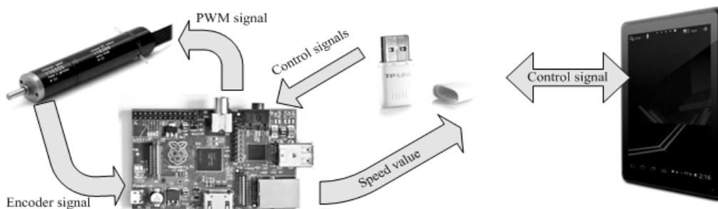
Fig. 3 Functional chart of developed control system
