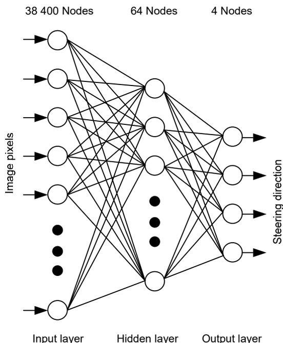
Fig. 6. Structure of implemented Neural Network
