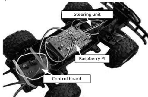
Fig. 2. The photo of the mechanical part with the installed Raspberry Pi-based control board
