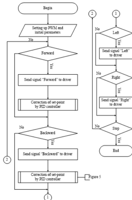
Fig. 4. Algorithm of RC car movement control
