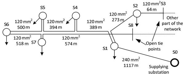
Fig. 7 Simplified layout of analysed MV network
