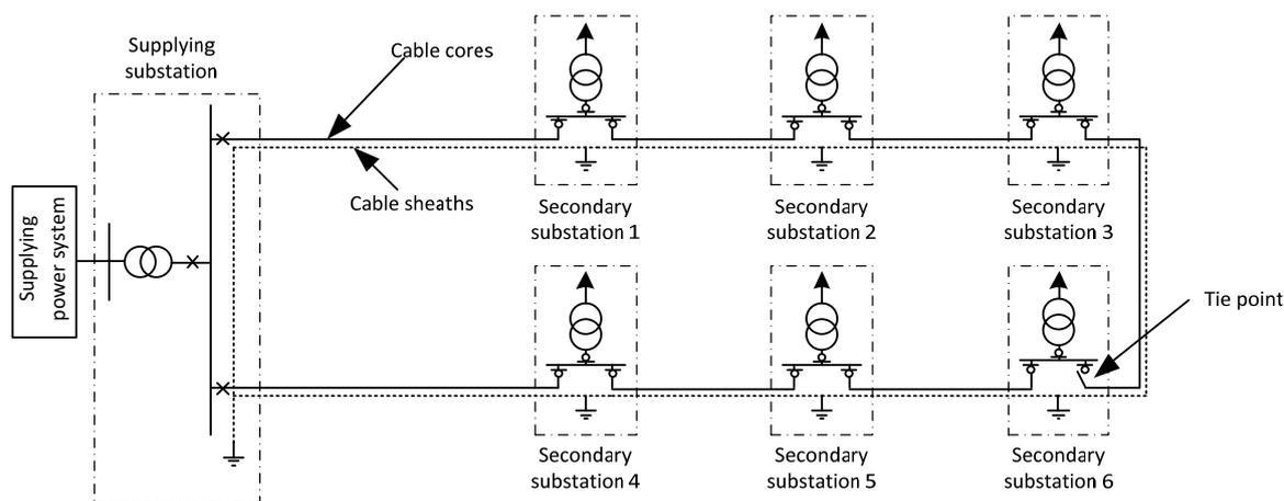
Fig. 1 Typical arrangement of medium voltage open-loop network
