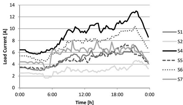
Fig. 8. Substation load profiles based on measurements
