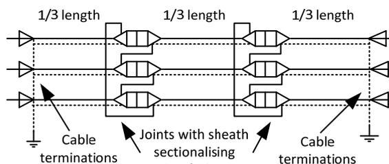
Fig. 3. Typical sheath cross-bonding
