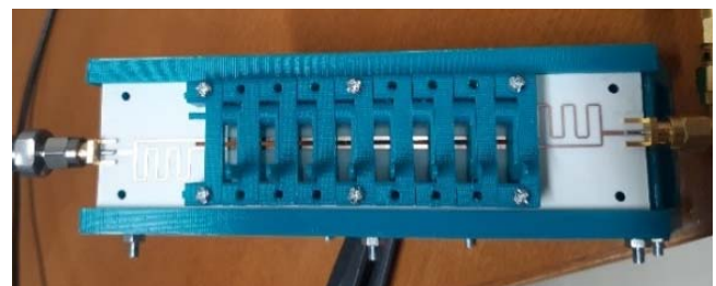
Fig. 10 Seed moisture measurement sensor constituting a transmission line
