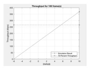
Fig. 5. The throughput 100 frames against the range of SNR -6 and 10 dB
