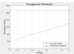
Fig. 1. Throughput for 100 frames against the range of SNR -2 and 2 dB  $\,$
