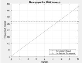
Fig. 4. The throughput for 1000 frames against the range of SNR -6 and 10 dB  $\,$
