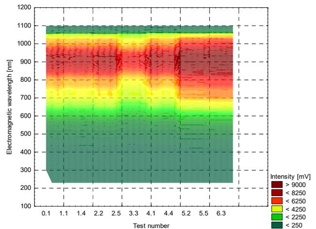
Fig. 8. Electromagnetic wavelengths identified after passing through a fluid with different plasma levels
