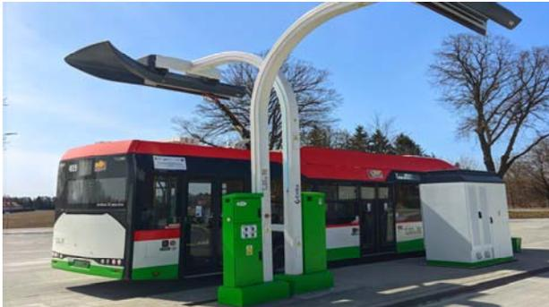
Fig. 2. The view of two charging stations and Solaris Urbino Electric 12 electric bus being charged
