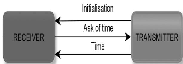
Fig. 3. Method of measuring distance by measuring the response time
