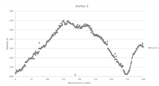
Fig. 11. Graph of ToF values for anchor 2
