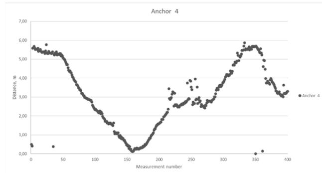
Fig. 13. Graph of ToF values for anchor 4
