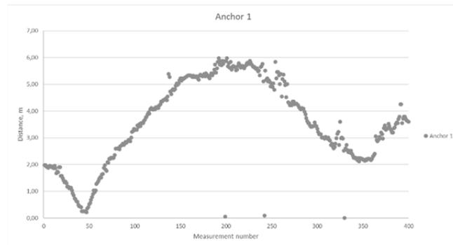
Fig. 10. Graph of ToF values for anchor 1
