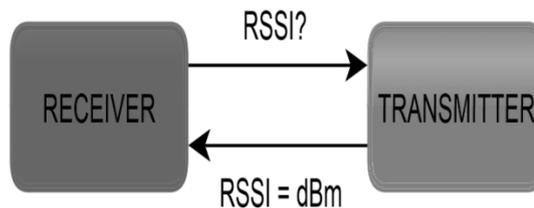
Fig. 1 RSSI measurement with response
