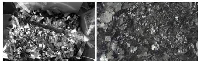
Fig. 1. Examples of base materials: a) nanocrystalline tapes, b) flake of iron scale.
