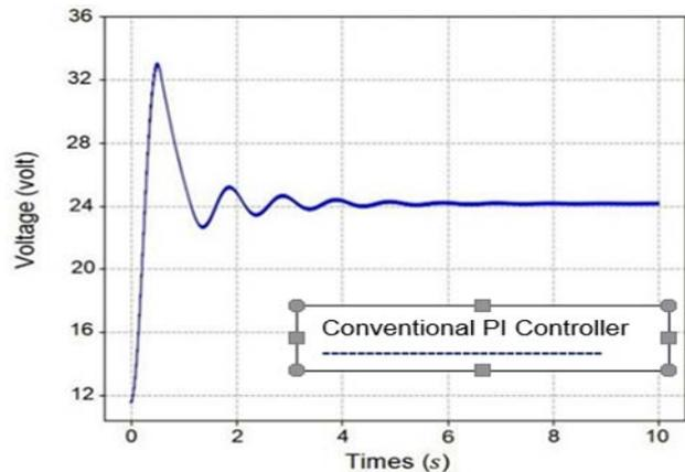
Fig 6. Conventional PI Controller simulation result of the output voltage DC-DC boost converter.
