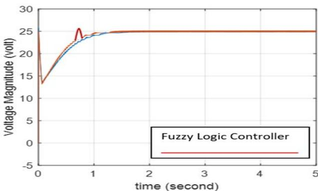
Fig 5. Fuzzy Logic Controller simulation results of the output voltage DC-DC boost converter
