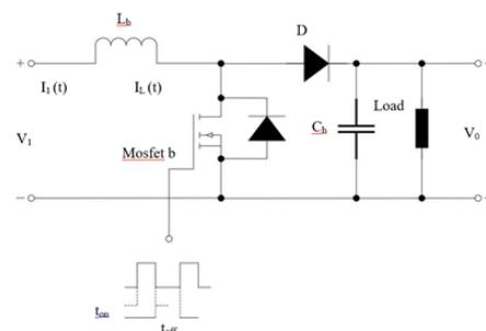
Fig 1. Circuit of DC-DC Boost Converter
