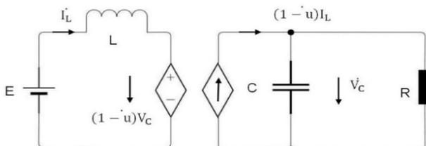
Fig 2. Equivalent circuit of DC-DC boost converter operating in ccm
