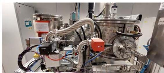
Fig. 1. Home made vacuum equipment for large area metallic electrodes deposition.
