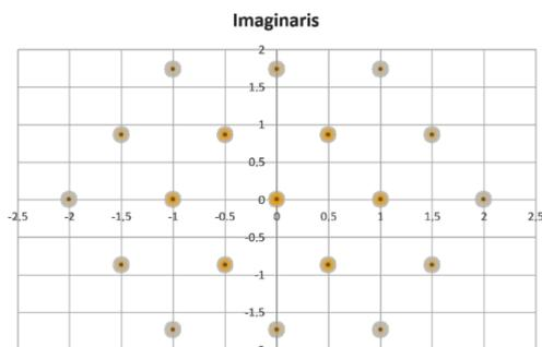
Figure 3. The polar voltage space vectors of the two-level six-phase VSI
