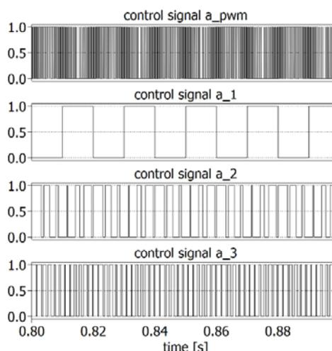
Figure 5. The comparison of the control signal waveforms for various control strategy and for phase a
