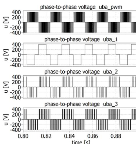
Figure 6. The comparison of the phase-to-phase voltage waveforms for various control strategies
