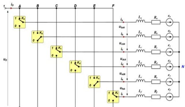
Figure 1. The model of the 6-phase 2-level inverter with the star connected load
