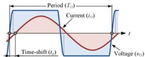
Fig. 3. The time-shift between  $v_O$  and  $i_O$ .
