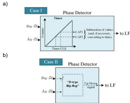
Fig. 2. Phase-detector operating principles.
