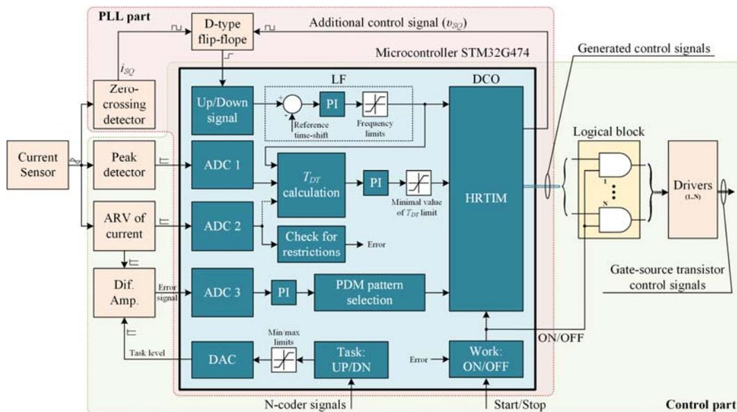
Fig. 8. The block diagram of the SRI control system.
