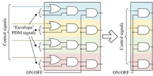
Fig. 7. Logical block simplification.
