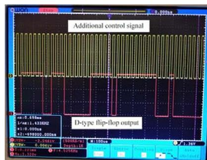
Fig.12. Changing the output signal of the D-type flip-flop in relation to the additional control signal.
