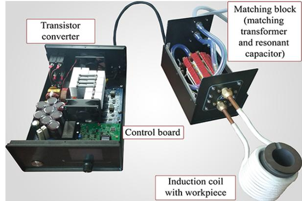
Fig. 9. The prototype of an induction heating system for melting applications.
