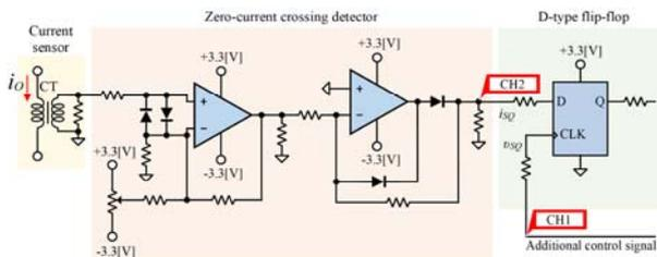
Fig.10. Circuit diagrams of some blocks of the SRI control system.
