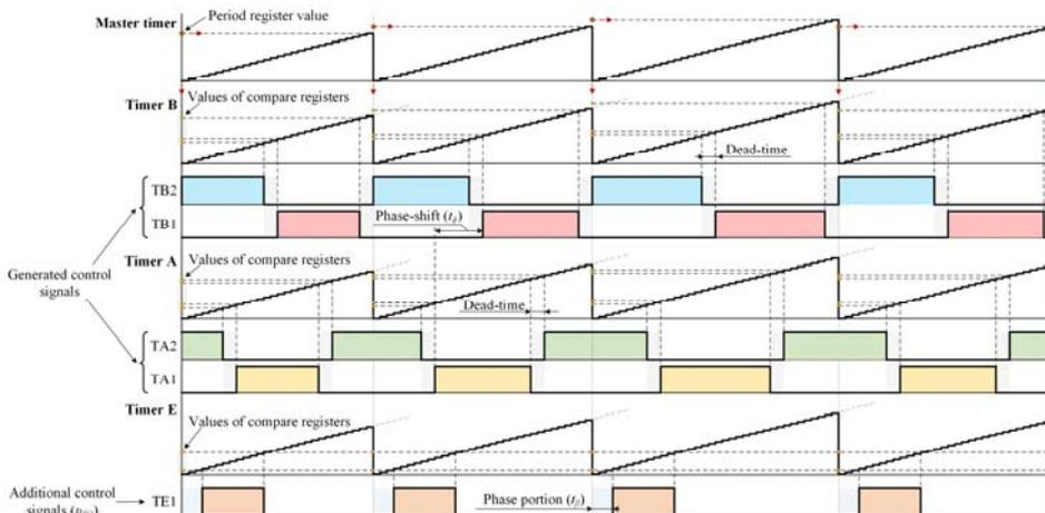
Fig.6. An example of generating control signals using the HRTIM for the PS control method.
