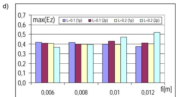
Fig.5. The influence of the diameter of the reinforcement on the  $\max(E_z)$  value with the conductivity  $\sigma=0.004$  S/m and the relative electric permittivity : (a)  $\epsilon_r'=5$ ; (b)  $\epsilon_r'=6$ ; (c)  $\epsilon_r'=7$ ; (d)  $\epsilon_r'=8$
