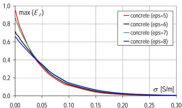
Fig.1. Changes in the  $\max(E_z)$  value depending on the conductivity for different values of relative dielectric permittivity
