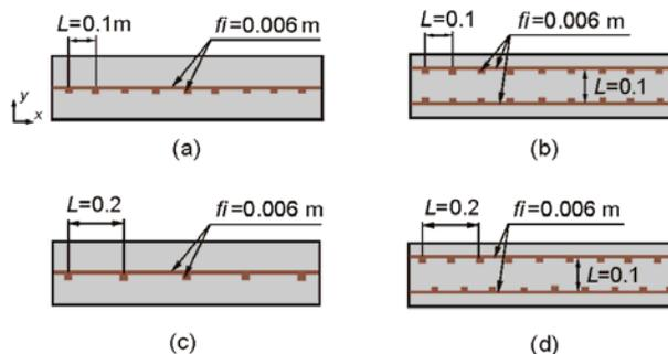
Fig.3. Variants of the analysed walls: (a) L10(1p); (b) L10(2p); (c) L20(1p); (d) L20(2p)
