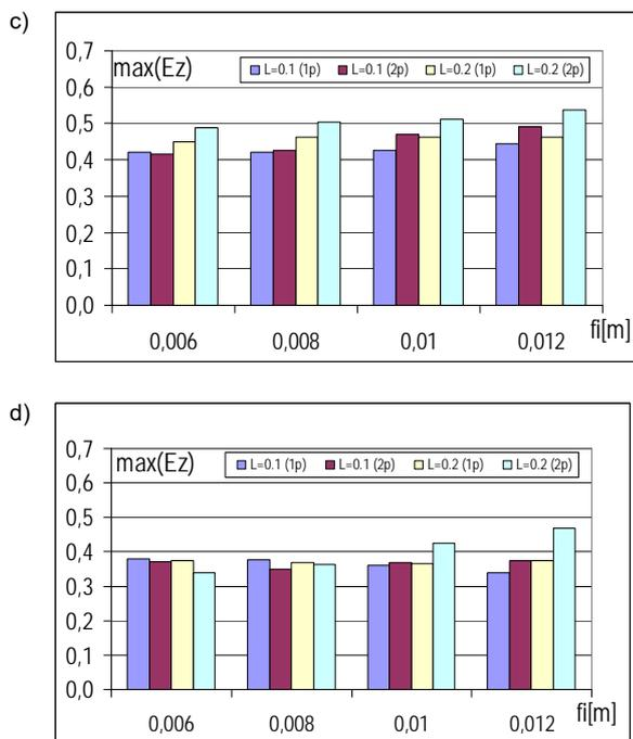
Fig.6. The influence of the diameter of the reinforcement on the  $\max(E_z)$  value with the conductivity  $\sigma=0.01$  S/m and the relative electric permittivity: (a)  $\epsilon_r'=5$ ; (b)  $\epsilon_r'=6$ ; (c)  $\epsilon_r'=7$ ; (d)  $\epsilon_r'=8$
