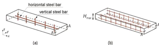
Fig.2. Three-dimensional view of the concrete wall model with reinforcement, where: A-A denotes the plane on which the field intensity distribution for the model was assessed: (a) 1p; (b) 2p
