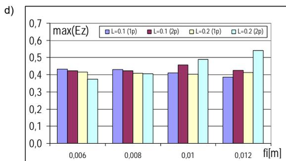
Fig.4. The influence of the diameter of the reinforcement on the  $\max(E_z)$  value with the conductivity  $\sigma=0.00195$  S/m and the relative electric permittivity : (a)  $\epsilon_r'=5$ ; (b)  $\epsilon_r'=6$ ; (c)  $\epsilon_r'=7$ ; (d)  $\epsilon_r'=8$
