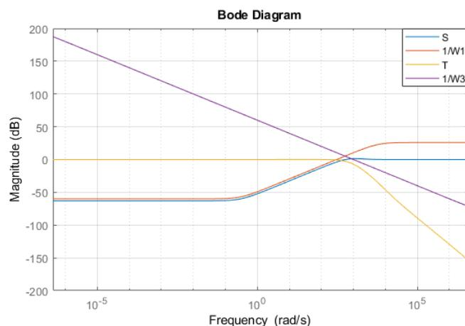
Fig.4. Bode plot of  $S$ ,  $\frac{1}{W_1}$  and  $T$ ,  $\frac{1}{W_3}$  for Hinf control
