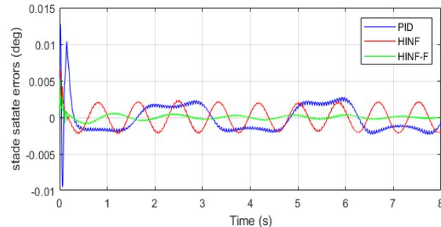
Fig.7.The state error for joint 1 ( $\mathcal{G}_1$ )
