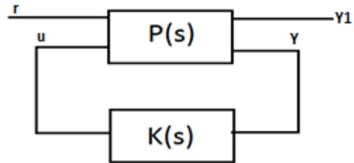
Fig.2. Closed-loop system
