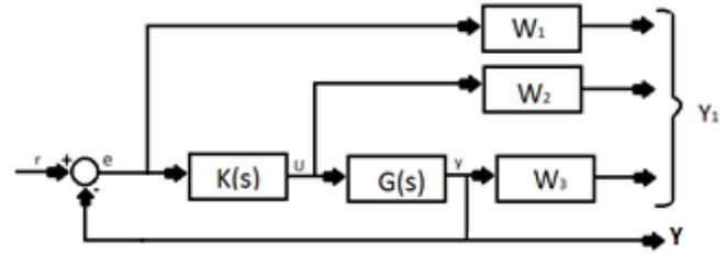
Fig.1. The augmented plane
