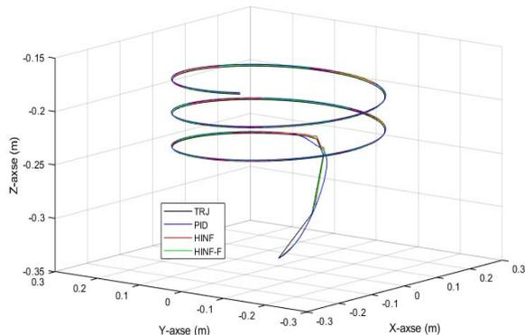
Fig.6.operational trajectory tracking under the proposed Controller
