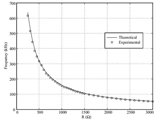
Fig.7. Frequency tuning of proposed single-phase oscillator
