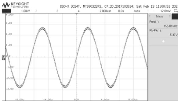
Fig.5. Sinusoidal waveform of a single-phase sinusoidal oscillator
