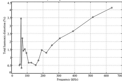
Fig.9. Total harmonic distortion of sinusoidal signals
