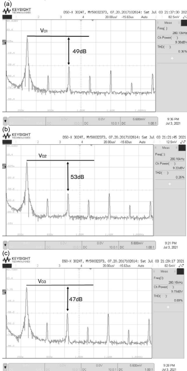
Fig.11. The experimental spectrum analysis results of the MSO (a)  $V_{01}$  (b)  $V_{02}$  (c)  $V_{03}$
