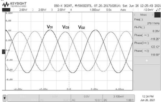
Fig.10. The output waveforms of the MSO
