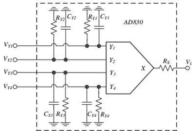
Fig.3. Parasitic elements of AD830
