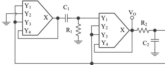
Fig.2. Proposed single-phase sinusoidal oscillator
