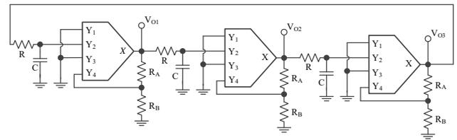
Fig.4. The proposed MSO circuit
