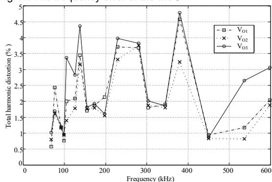
Fig. 15. The total harmonic distortion percentage of the MSO
