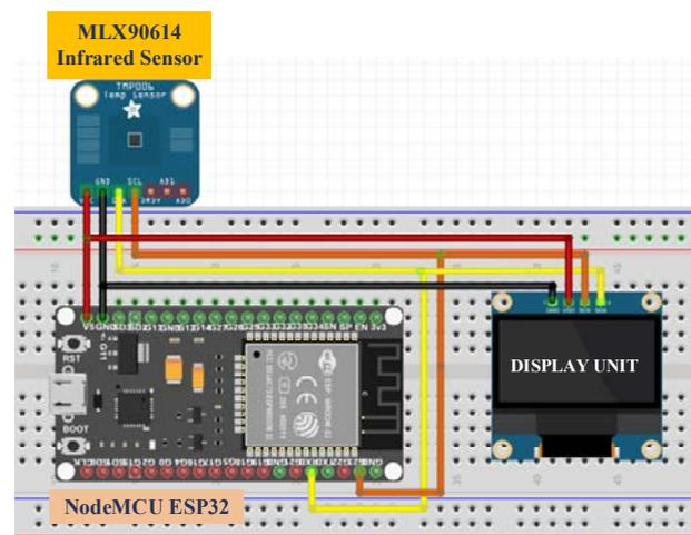
Fig.2 Schematic circuit of the hardware device
