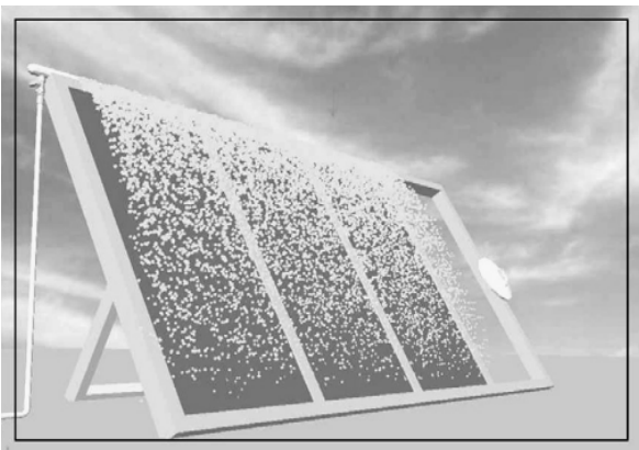
Fig 2. Transmitting water from the pump to over the front of the cells [12].
