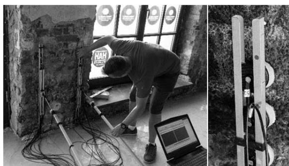
Fig. 1. EIT test stand: (a) - measurement site, (b) - electrode approach, (c) - electrode structure.
