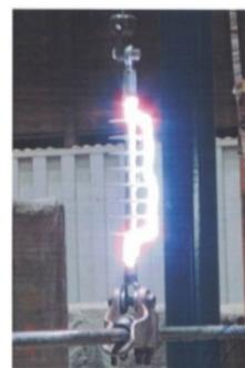
Fig.15. Lightning Impulse Wet flashover voltage test
