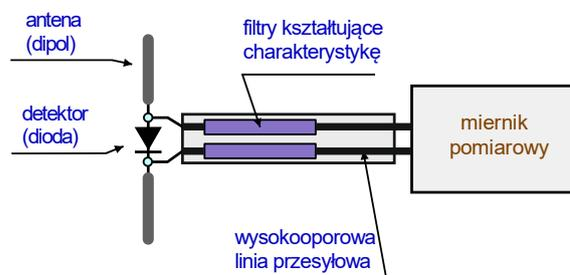
Fig. 4. Measuring diode with a diode detector [1].
