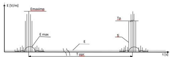
Fig. 2. Time and amplitude dependencies of pulsed radiation at the measuring point during irradiation measurement by a radar device
