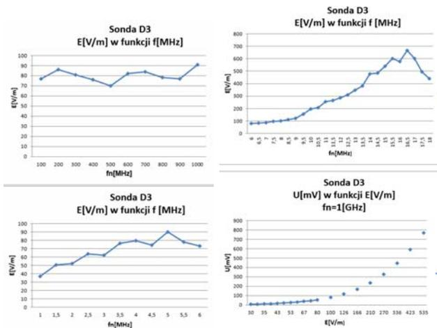
Fig. 8. Test results for measuring probe elements sonda D3 – D3 probe; E[V/m] w funkcji f[MHz] - E[V/m] as a function of f[MHz]
