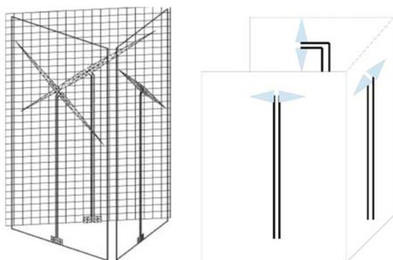
Fig. 3. Arrangement of receiving antennas within a probe (regular triangular prism, regular rectangular prism)
