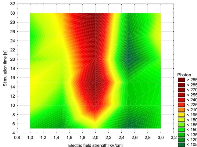
Fig. 9. Photon emission structure as a function of electric field strength and stimulation time
