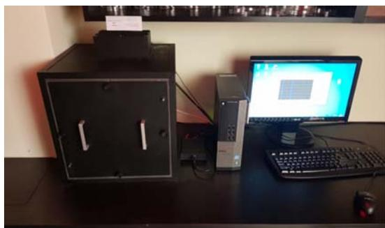
Fig. 3. Test stand for single photon counting
