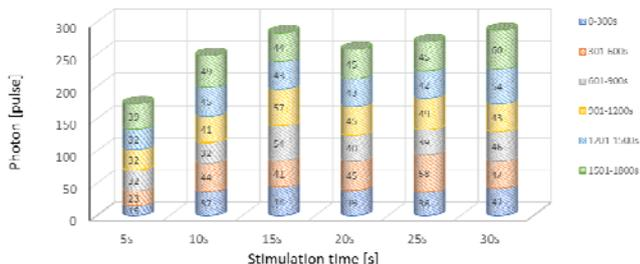
Fig. 6. Photon emission structure of oilseed rape seeds after stimulation with 2 kV/cm electric field
