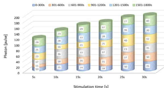
Fig. 5. Photon emission structure in rapeseed after stimulation with 1.5 kV/cm electric field.
