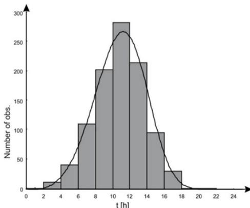
Fig. 9. Empirical distribution determined by simulation for 1000 generated values according to Weibull (bar chart) and theoretical (solid line) distribution
