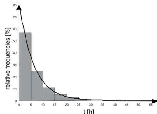
Fig. 3. Empirical distribution determined by simulation for 1000 generated values according to exponential (bar chart) and theoretical (solid line) distribution
