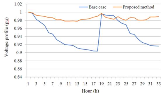
Fig. 2. Voltage profile for base case and Reconfiguration by the installation of DG units and capacitors for 33 node test system
