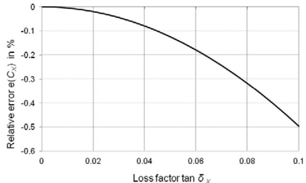
Fig.4. Relative error  $e(C)$  vs. measured loss factor  $\tan \delta$
