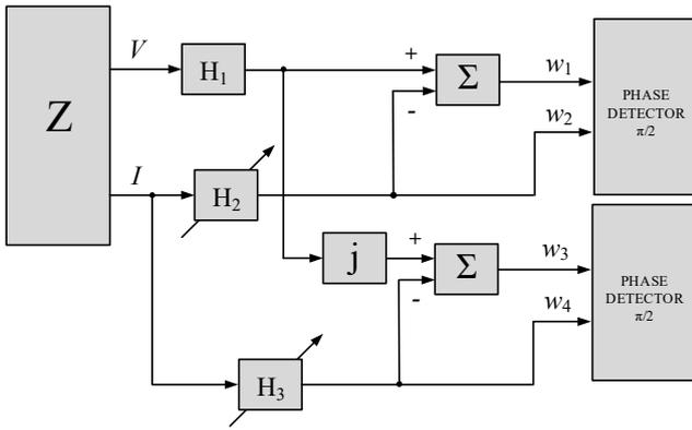
Fig.2. Schematic diagram of the parallel quasi-balanced circuit
