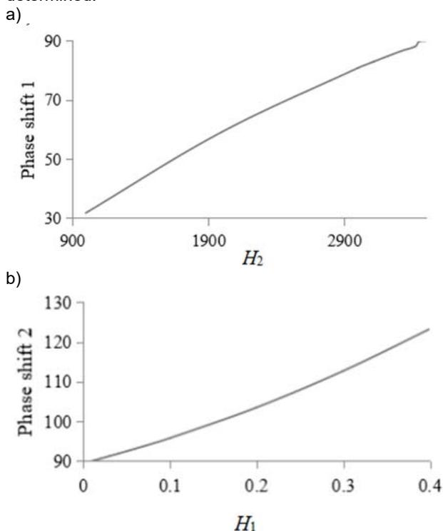
Fig.10. Dependence of the output signals (phase shifts) vs settings of the adjustable elements  $H_1$  and  $H_2$
