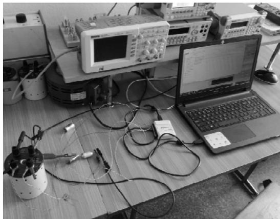
Fig. 9. View of the implemented system for measuring the dielectric loss factor  $\tan \delta$
