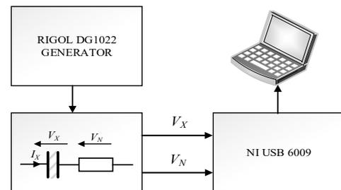
Fig.6. Simplified schematic of the virtual measuring circuit
