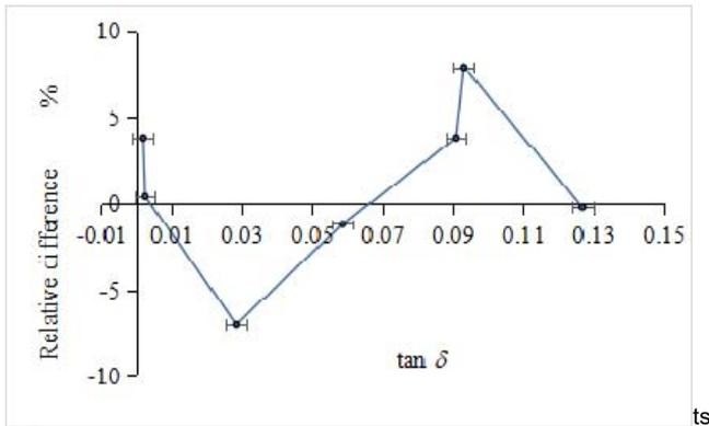
obtained with circuit shown in Fig. 3 and results of  $\tan \delta$  measurements made with a commercial LCR meter. Bars represent standard uncertainty of the measurement ( $k = 1$ )
