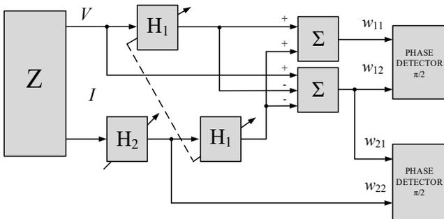
Fig.3. Schematic diagram of circuit with dual quasi-balancing
