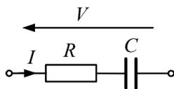
Fig. 1. A simple model of the impedance of an electrical insulator
