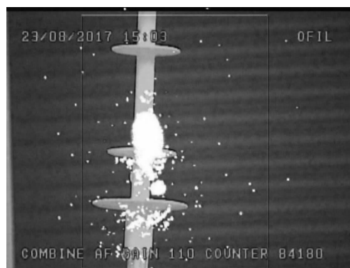
Fig.2. Example photo of an insulator during UV camera testing. Source: own study
