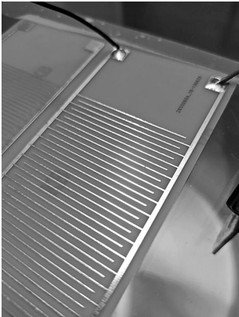
Fig. 2. Electroadhesive pad with comb-shaped electrodes
